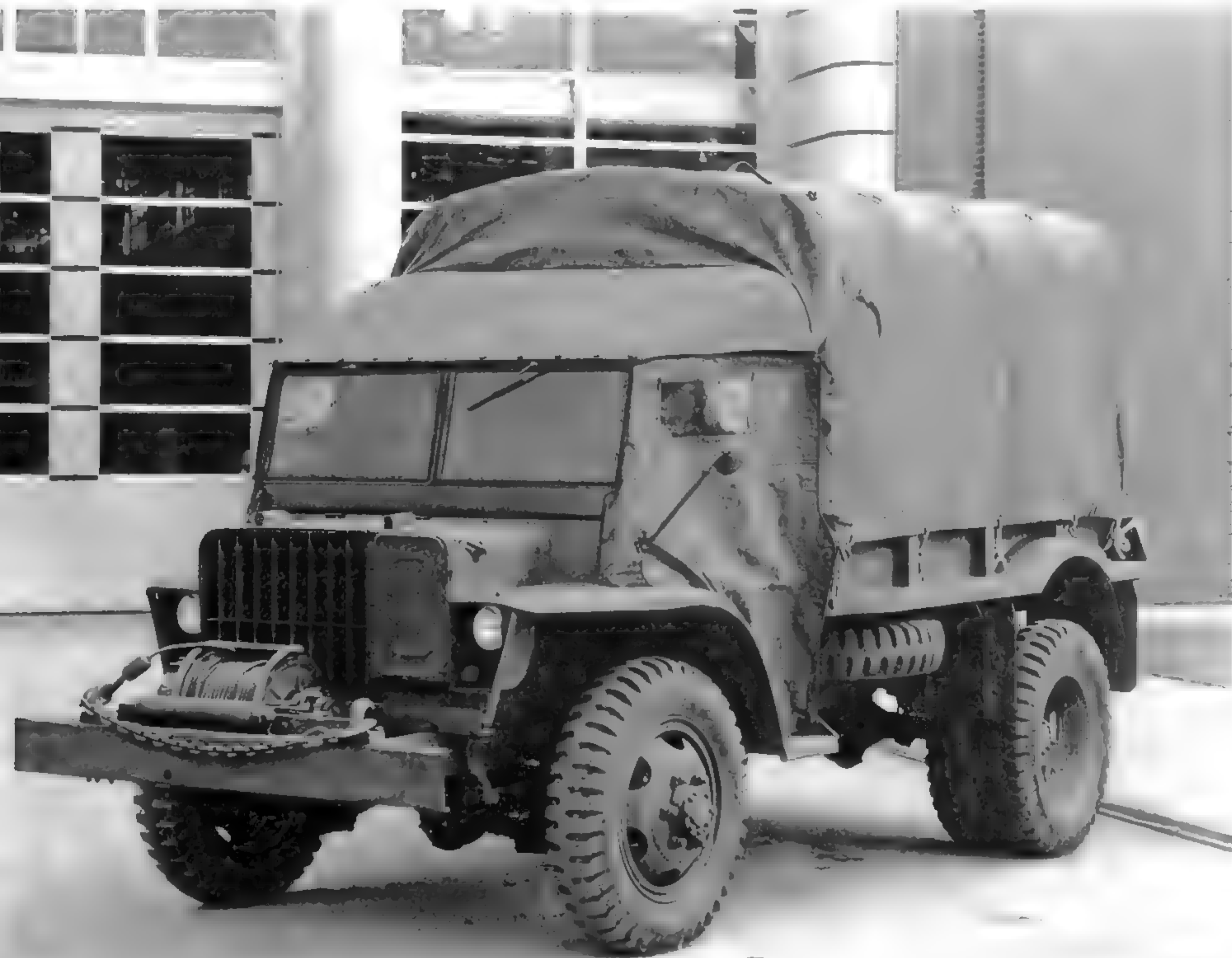
The GTBS was the first variant used by the Navy for a bomb service truck. In this photo the single rear tires characteristic of the GTBS are visible. This truck lacks a front winch. (Photo courtesy of the Bryce Sunderlin collection)
